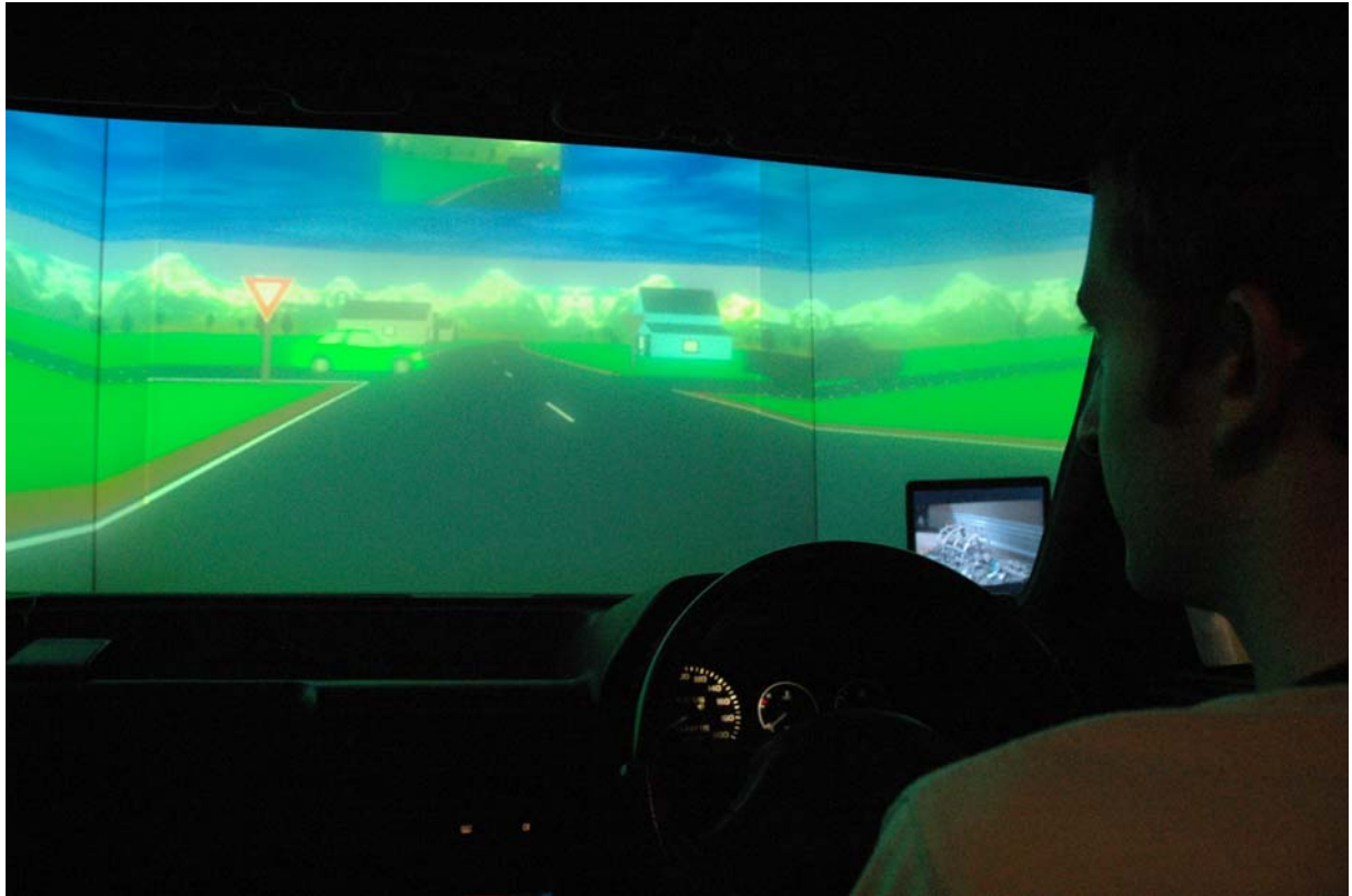
Figure 2: Simulator car body, screens, and laptop PC presenting visual materials
